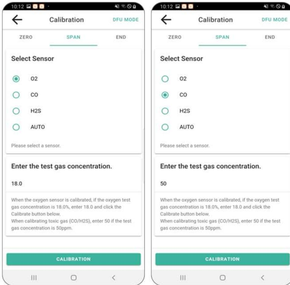
Span calibration can be performed for each sensor as shown above, or all sensors can be calibrated in batches by pressing the Calibrate button after selecting AUTO. concentration of test gas used for calibration is set as shown in the following table.
