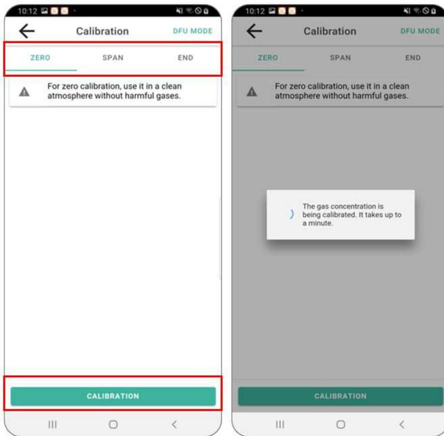
If you enter the gas concentration calibration page in the dedicated app, you can see that there are 3 types of menus such as “Zero Calibration”, “Span Calibration” and “Complete” on the upper part. After selecting the **Zero Calibration** menu, press the Calibrate button and the gas concentration calibration will start as shown in the figure on the right upper part.
